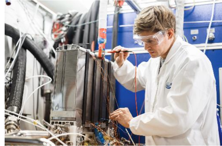
100 kW automotive fuel cell stack on ZSW test bench
