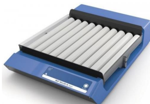
FIGURE 2: ROLL MILLER (IKA ROLLER 10 BASIC) USED FOR INK HOMOGENIZATION
