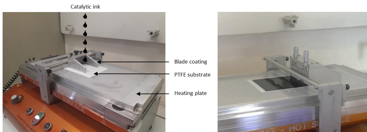
FIGURE 3: ELCOMETER BLADE COATING EQUIPMENT
